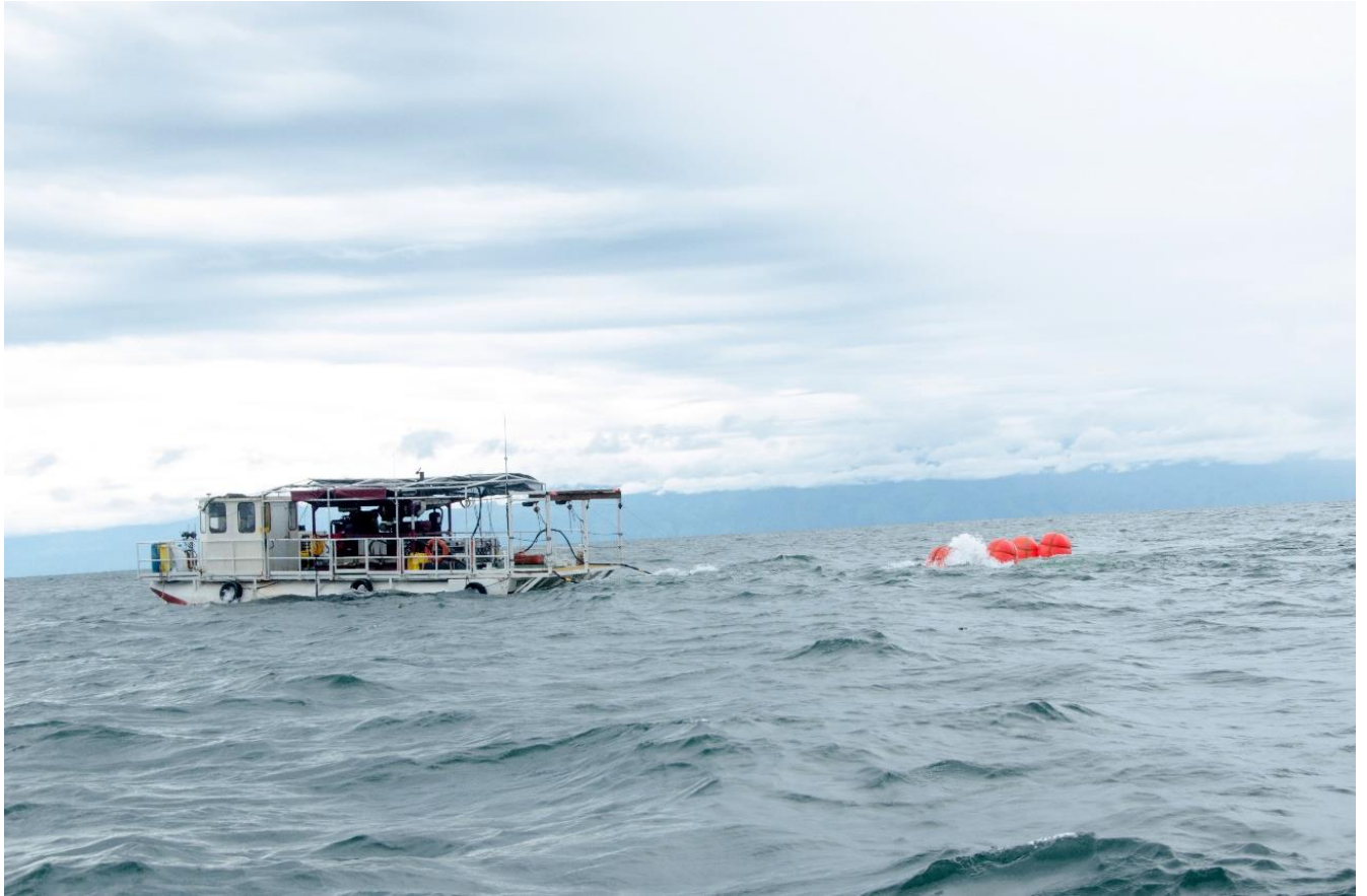
5) Airguns (right) in action on Lake Albert. Airguns are vital equipment in the 2D seismic data acquisition exercise.
